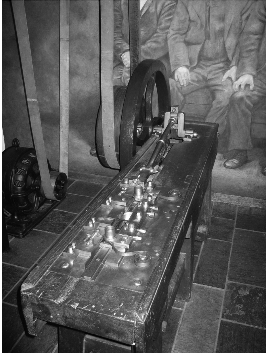
Fig. 4. Double milling machine from the nineteenth century; probably built 1813-14 in Kongsberg, Norway. Norwegian Mining Museum, Kongsberg. Photo by Frode Sæland. See Cooper 1988, p. 194.
