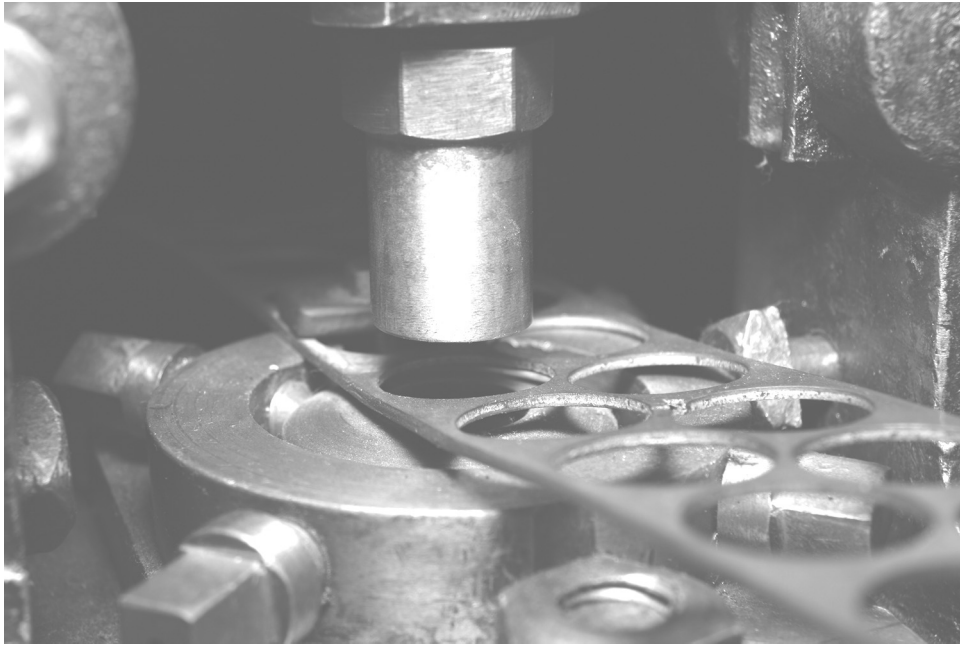
18) Punching out planchets from strip. Mounting at Norwegian Mining Museum. Photo: Christian Berg.
